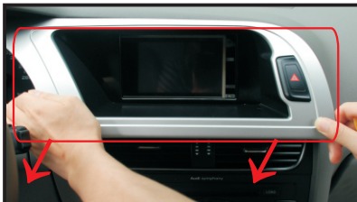
3.Take out the decoration plates, pay attention to the buckles and connection
