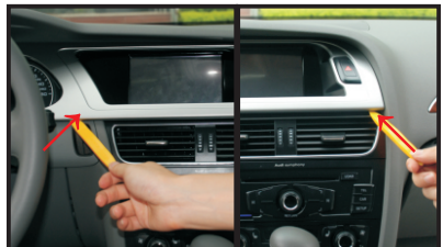
2. Use plastic pry to pry decoration plates as the picture show
