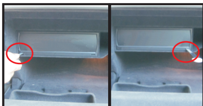
13. Take out the outside box of Multi-media with hardware key, pay attention to spring plate (The normal mode and comfortable mode without this step )
