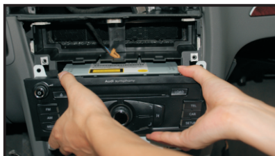
12. Take out original host and disconnect those cables
