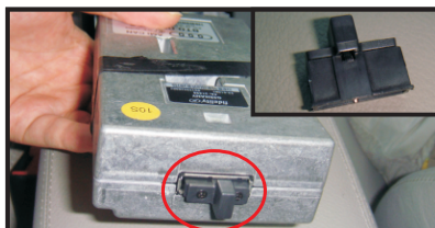
20. Put multi-connection plug into the original Multi-media box, pay attention to the direction (the normal mode and comfortable mode without this step)
