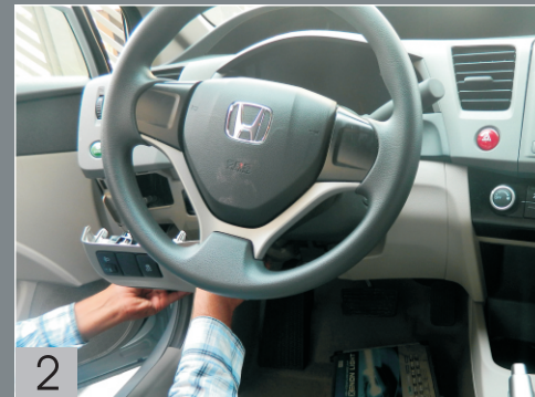
2 Pry the left panel below the steering wheel.
