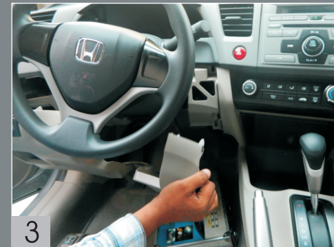
3 Pry the right panel below the steering wheel, then take it out.
