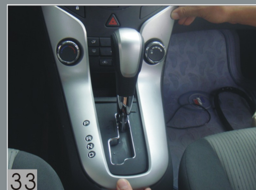
Install the decorative plate and note each buckle and wiring connection.
