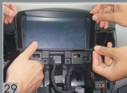
Connect the wiring of the screen of GPS device, then install the screen to the car. Fix the screws and note the buckles.
