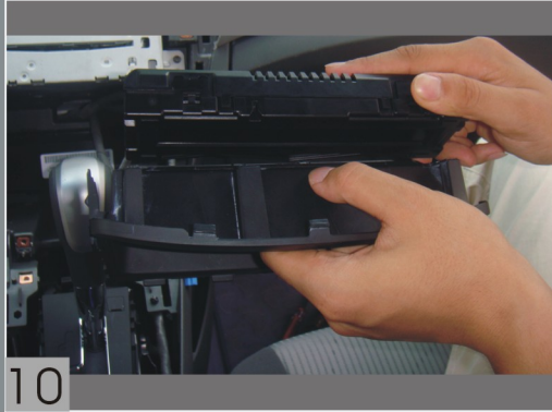
Remove the original car screen from screen frame and note each buckle.
