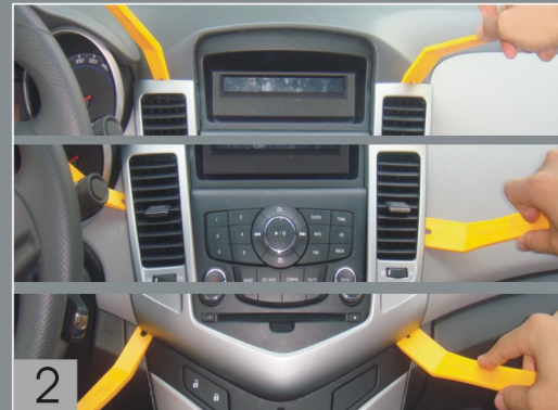
Pry the air-condition outlet frame with crow plate and be care of buckles.
