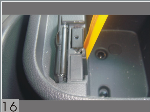
Pry the original car AUX socket with crow plate.
