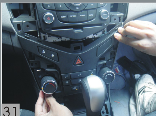
Connect the wiring of the air-condition panel and fix it to the car.
