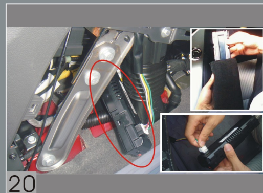
Package the screen of original car with protection kit and connect wiring harness. Install the screen to the place as picture show and fix it well.
