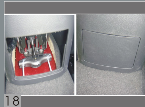
Connect the two plugs. Please keep wires in order to avoid the effect to the handbrake function. Install the cover panel of glove box.
