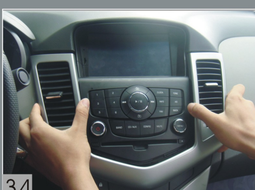
Install the decorative plate of air condition air outlet and note each buckle.
