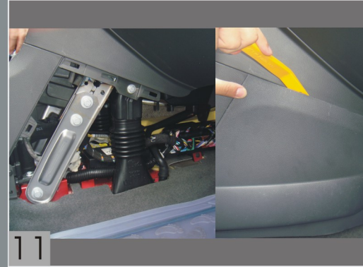
Remove the left guard plate from the position of copilot and note each buckle.
