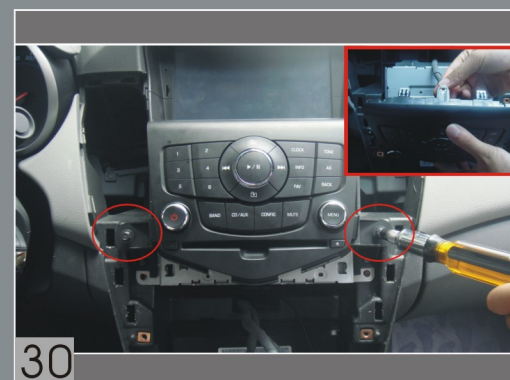
Connect the wiring of the head unit panel, then install it with screws.
