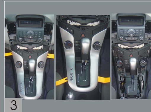
Pry the decorative plate of gearbox with crow plate. Be care of buckles and wiring.
