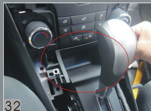
Install the gearbox and fix the screws on the air-condition panel.
