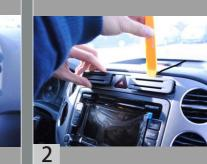
Pry the right air-condition outlet with crow plate as shown in the picture.
