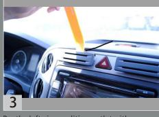
Pry the left air-condition outlet with crow plate as shown in the picture.
