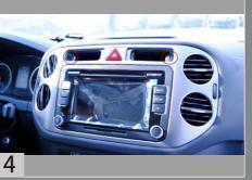
Remove the four screws used for fixing air-condition.
