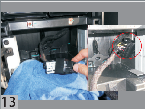
Connect the transfer cable and put it in the gap at the right side.
