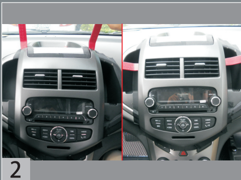
Remove the frame panel with special tools.
