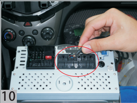
Connect all the connectors in the box.
