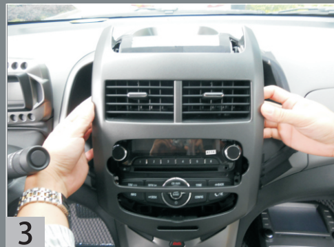
Take apart the frame panel carefully.
