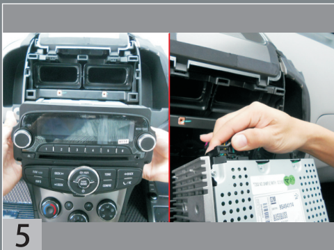
Take the radio out and unplug all the plugs behind it.
