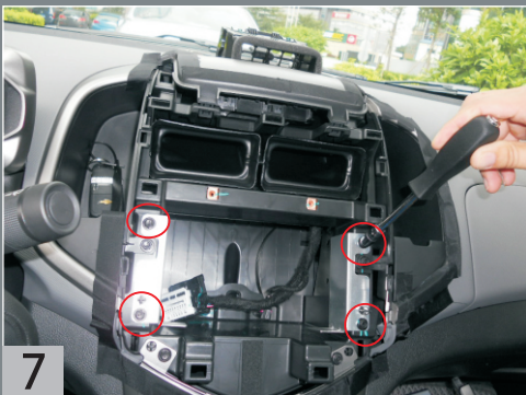
Put the brackets A&B in the right position and fix them with screws.
