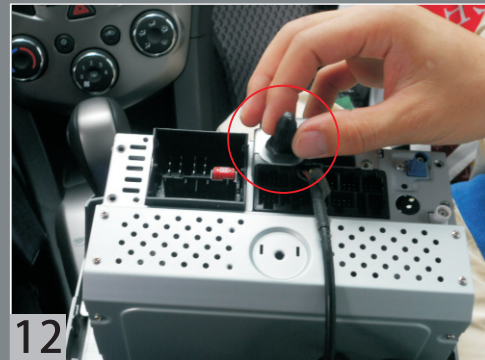
Remove the fixing pole of original radio and install it on the navigation system.
